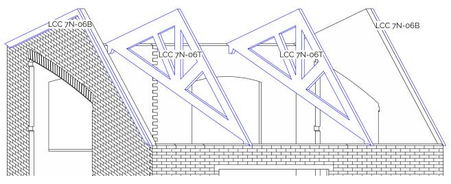
Trim the roof panels to width. Measure twice cut once. The height of LCC 7N-06R is designed to fit this kit with a little bit of overhang. It can be reduced by trimming the panel to height.
