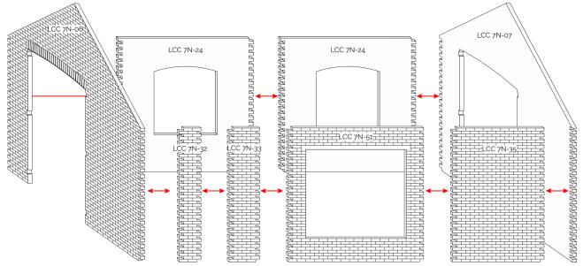
The inner deck and platform side were designed such that the goods shed can be made longer if needed. They need to be trimmed for this building. Note the sliding gate opening is not in the centre and that needs to be accommodated for when measuring.
